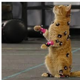
Figure 8. Mocap sensors on a cat to record its movements.
