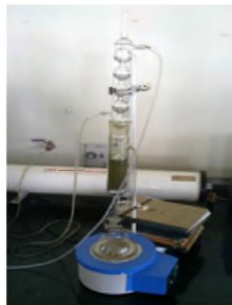
Fig 2: Soxhlet extraction of leaf and bark samples of Annona muricata by different solvents
